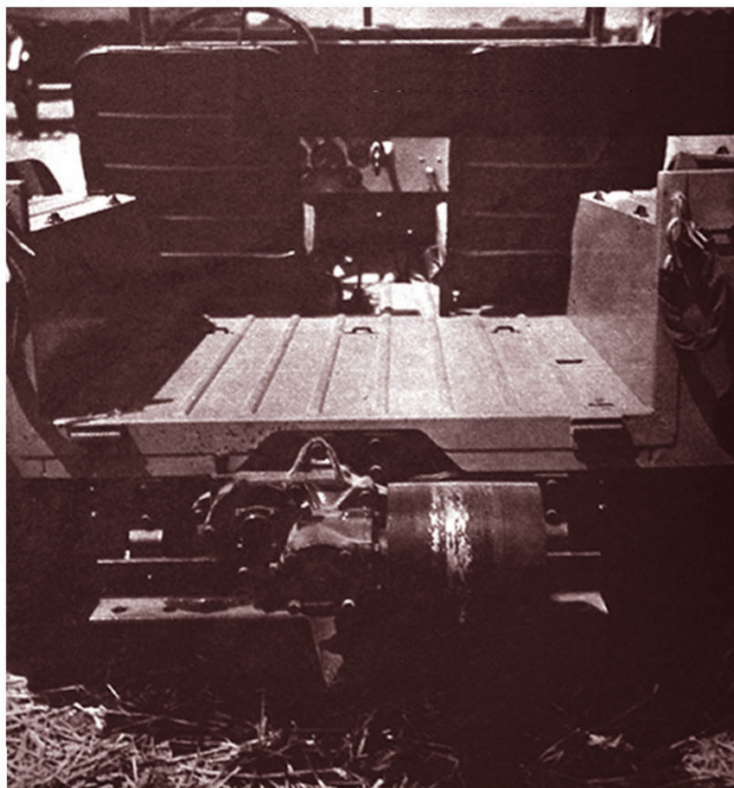
Here, with jeep's tail board down, is the power attachment, to make milk-shakes or cut trees.
