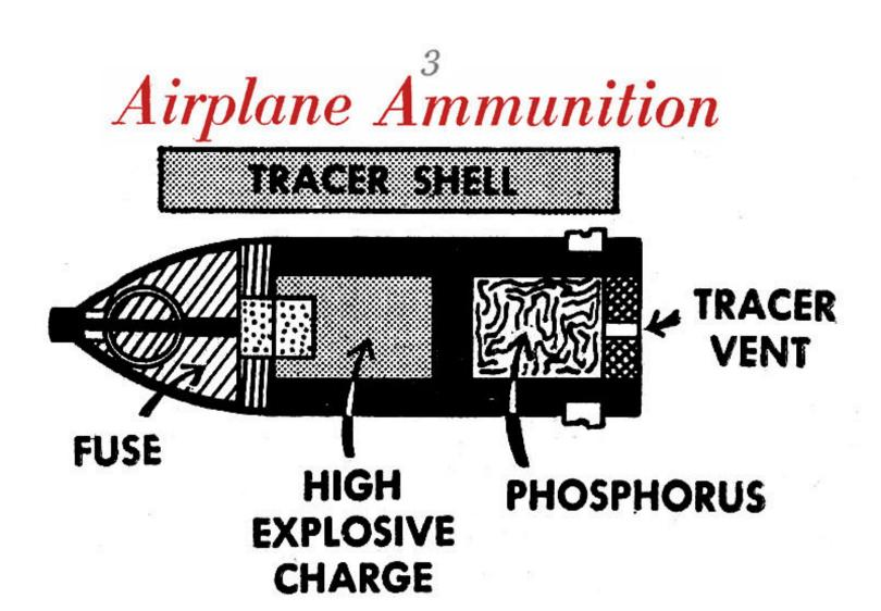
partment normally containing the high-explosive charge, and by filling the rear compartment with a suitable chemical, for example phosphorus. The tracer compound is set afire in the barrel by the heat of the powder gases and, spurting out through the vent, shows the line of flight. A day tracer produces mainly smoke, so that the trajectory appears as a dark smoky line, while a night tracer produces mainly fire, so that the trajectory can be seen as a luminous line against the dark background.
