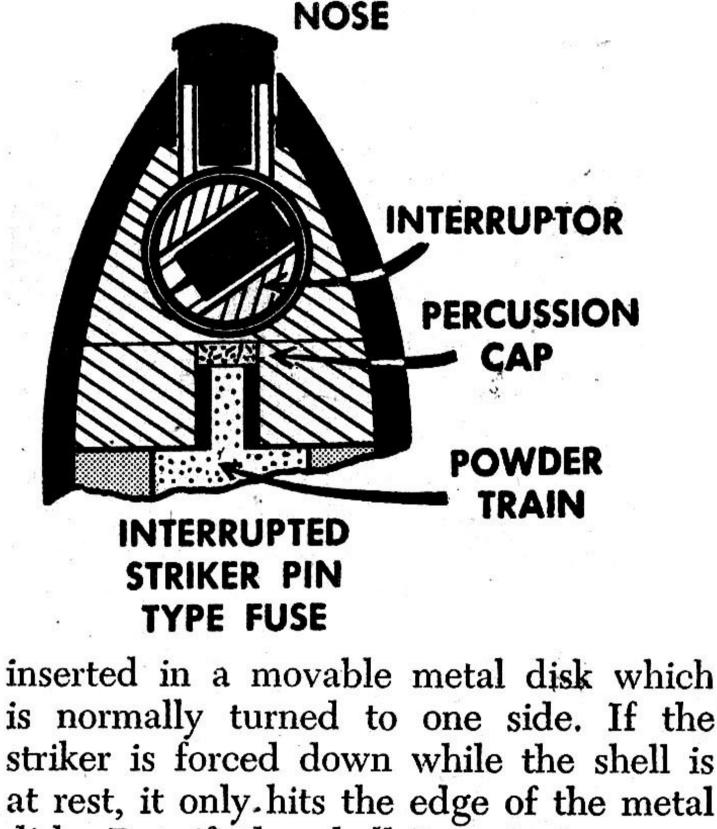
disk. But if the shell is spinning, centrifugal force has turned the metal disk around, so that the two parts of the pin are lined up. Just as ingenious and simple as the fuse constructions are the metal links that have replaced the old machine gun belts. Originally cartridges for machine guns were inserted in belts. It had the advantage that the belt could be refilled, but
