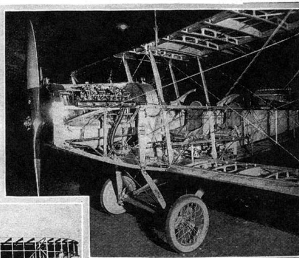
The covering of one side of this Curtiss two-seater has been cut away to show the complete construction and the passenger arrangement inside
