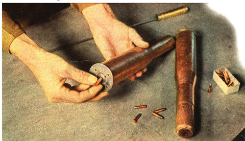
The Gunnery Dept. practices economy in target shooting by loading 37~m.m. shells ($4.35) with .22~cal. cartridges (less than a cent each)
