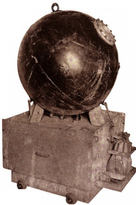
The mine unit is composed of a spherical sheet metal shell, containing a 300-pound charge of T.N.T. and a cubical box which is a combination anchor and housing for mooring gear.
