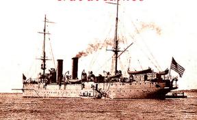
The mine layer San Francisco. The mines are launched from the stern. This stern, peculiar to mine layers, is clearly shown in this picture.
