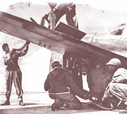
ARMORERS LOAD P-40 with .50-calibre ammunition and guns which give this plane its fearful, converging fire. Bullets go in tops of wings, guns are inserted from below. Crew here belongs to 96th Service Group, which maintains Oscoda fighter group's ships.
