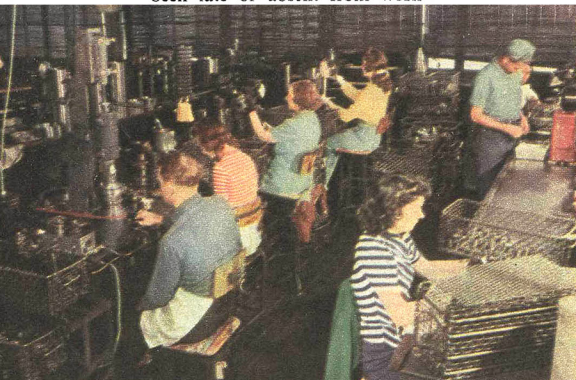
At a steel-testing machine, Dorothy (at rear) checks about 4,000 roller-bearing cones a day
