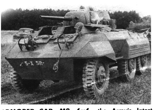
ARMORED CAR, M8, 6x6, the Army's latest combat vehicle, is a six-wheeled, eight-ton armored job that can hit high speed over practically any type of terrain. It mounts a 37-mm cannon and a .30-caliber machine gun in a hand-operated traversable turret. The M8 carries a crew of four and is intended primarily for use in reconnaissance combat.
