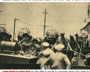
SUBMARINE-ELIMINATOR on the left is ready to proceed down the river to the Gulf of Mexico to clean out southern submarine nests. The round cans on the back are depth charges filled with a new ultra-powerful explosive. The 50-mm. turret machine-guns are also manufactured by Higgins.
