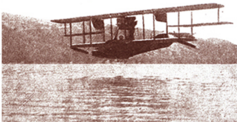
A four passenger Curtiss flying boat, the last word in airboat construction. This machine has a wing spread of 41 feet, is equipped with a 100 h.p. motor, and has a speed of 70 miles an hour
