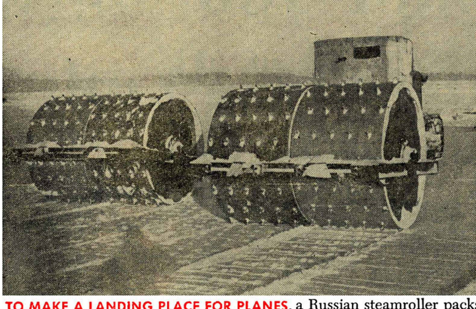
TO MAKE A LANDING PLACE FOR PLANES , a Russian steamroller packs down the snow. The spikes on the roller provide traction. This photo was taken in January, but it and most of the other pictures on these pages arrived just last week.
