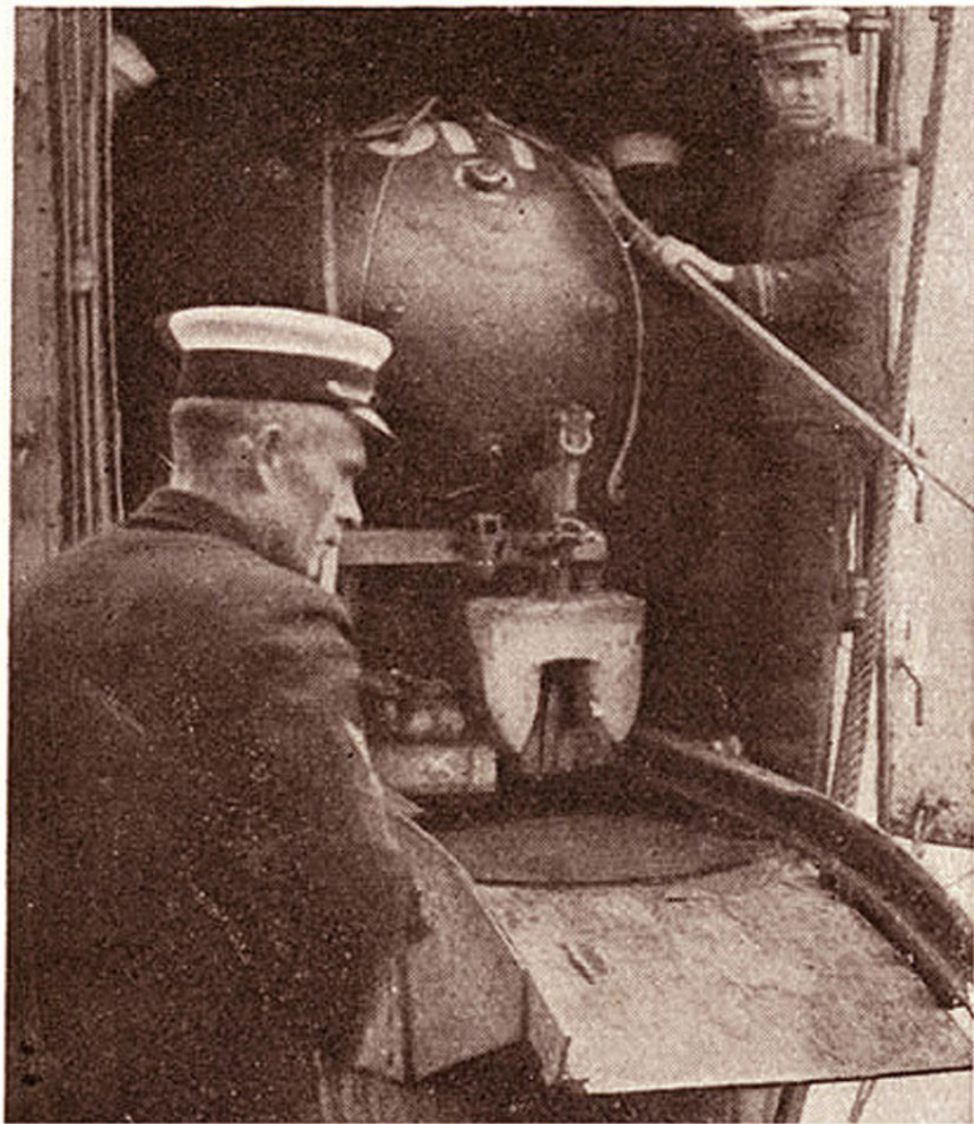
Taking the mine on board the mine layer. The mine is run in on a track.
