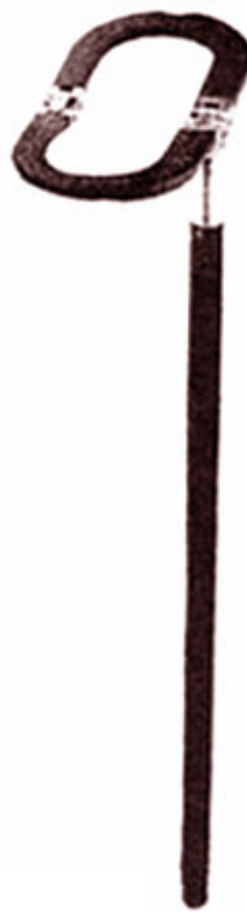
(D) The crooked handle of the stick shown in A opens to afford a seat and can be dug into the earth
