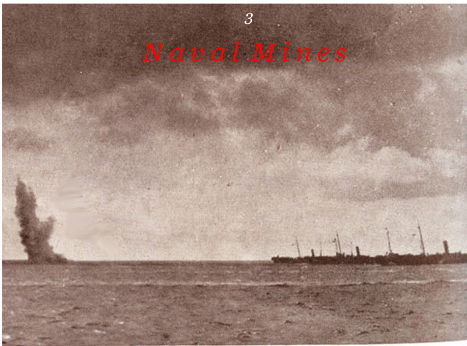
Destroying a defective mine. When a mine fails to submerge and anchor, a rifle shot from a destroyer removes the menace to merchant ships.
