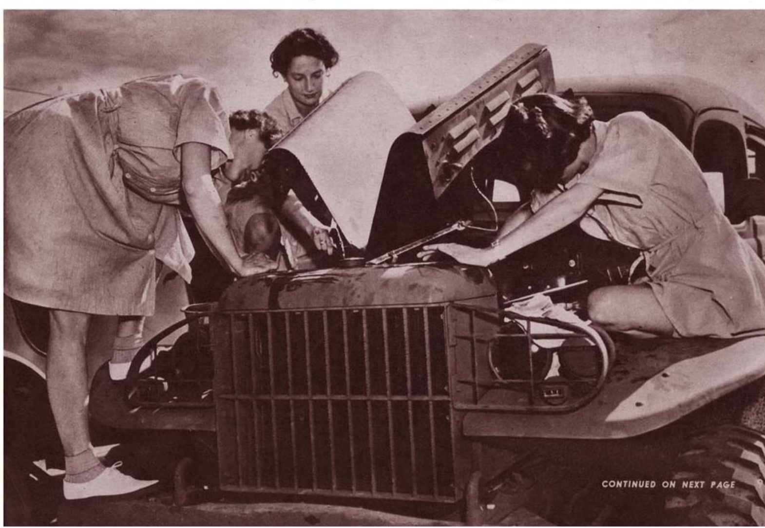
TAUGHT MOTOR REPAIR AND MAINTENANCE IN A SPECIALIZED CORPS FOR AUXILIARIES, THESE GIRLS WASH ENGINES WITH KEROSENE PRIOR TO INSPECTION
