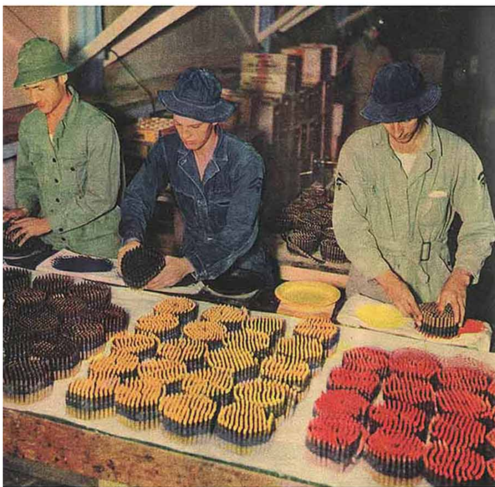
MACHINE-GUN BULLETS are dipped in specially prepared, vivid paints to stain the target. A different color is assigned to each gunner, so that his score can be controlled.
