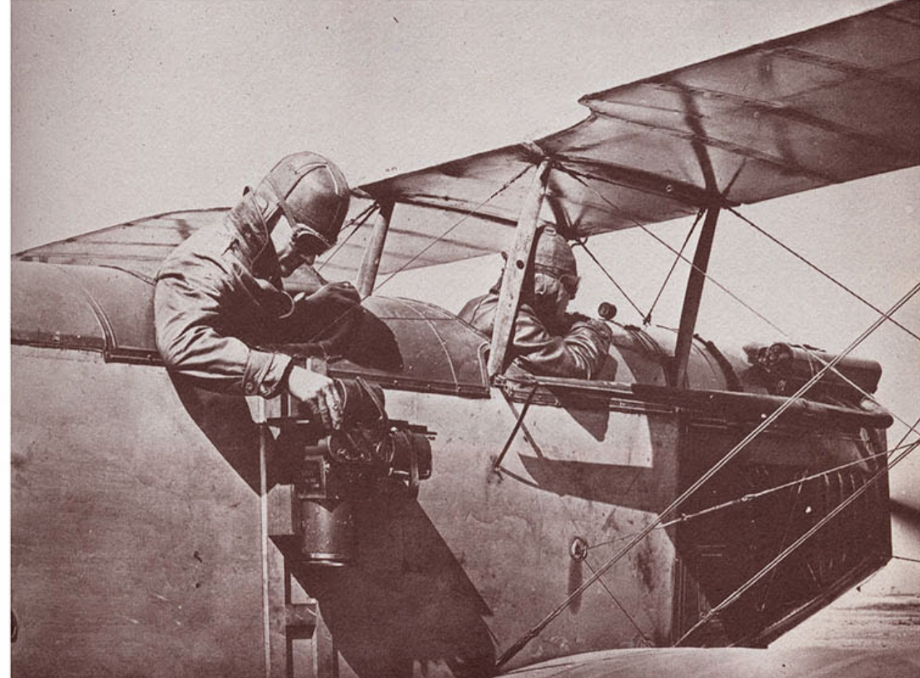
Method of attaching a camera to an airplane. The pilot is sitting in the front seat, and can operate the camera at the same time as the machine
