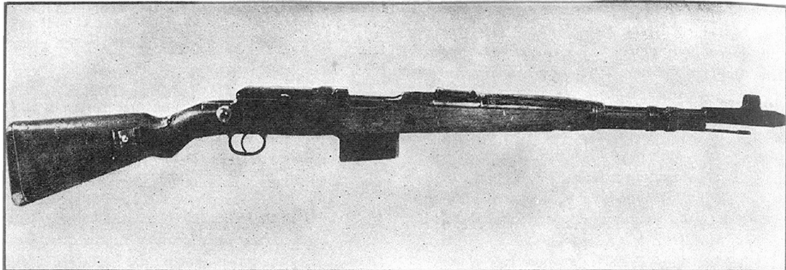
Figure 10.—Gewehr 41, caliber 7.92 mm semiautomatic rifle.
