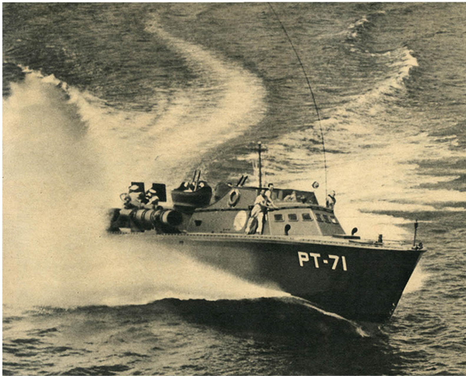
LATEST HIGGINS TORPEDO BOAT GOES OVER 50 M. P. H., CARRIES FOUR TORPEDO TUBES, TWO 50-MM. ARMOR-PIERCING GUNS, EIGHT DEPTH CHARGES, RADIO, SMOKE SCREEN DEVICES. HARD-HITTING "PT'S" ALREADY HAVE SUBS TO THEIR CREDIT.
