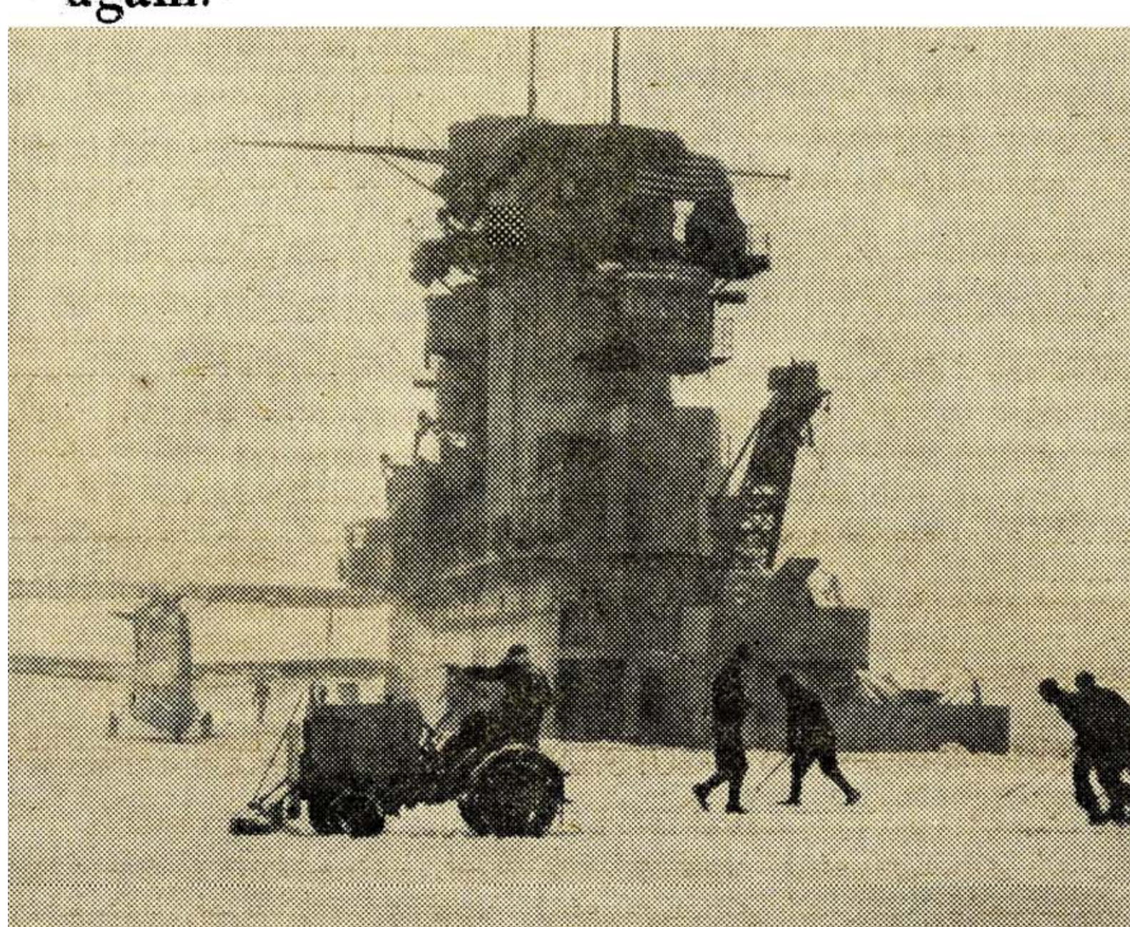
A SNOWPLOW is part of a carrier's equipment for clearing the deck on Winter patrol duty. Blizzards, fog and stormy weather hamper flying operations, and carrier must depend on speed and its destroyer escort for protection.
